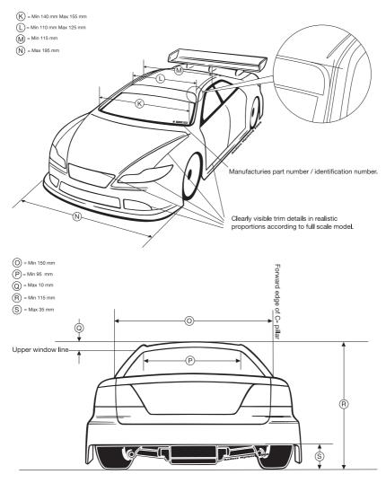
To assist competitors maintain consistent heights when using different wheels/ tyres, dimensions R and S will be measured with the chassis on a 15.0 mm block. Dimensions will be based on a 5 mm ground-clearance and will therefore be :- R = 125 mm, S = 45 mm.
