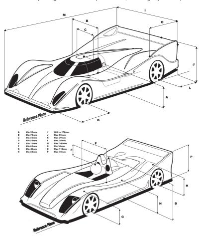
boxes) Minimum cockpit width – Closed cockpit – 70mm (Measured at the point it intersects with the side pod)
